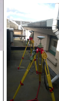
Checking the GPS kits on the roof
